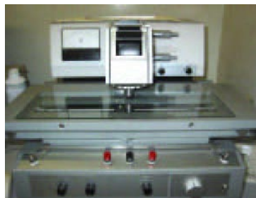
Scan the film with a microdensitometer
