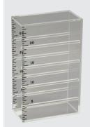
Test units can be set in the aluminum supporting box at 10, 15 or 20 mm (0.4,0.6 or 0.79 in) height
