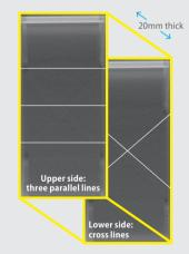
For verification of the spatial interval in reconstruction Stainless steel line: 0.1 mm/0.004 in dia.
