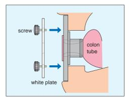
• Attach the white plate to the base so that the manual pump air tube fits in the notch. Affix the plate with the four screws.
