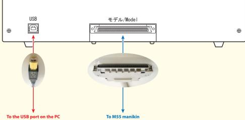
Shown above is the ports on the side of the USB box. Take note the direction of M55 manikin connector.
