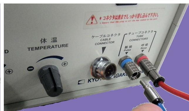
Matching the arrow of control cable end with the triangle on the port of the control box, connect the cable and port.
