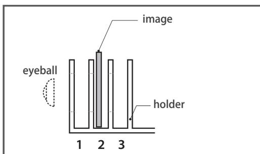
The first slit from the left is for simulating hyperopia (1) and the second slit is for simulating normal (2) and the third slit is for simulating myopia (3). (Please refer to the picture.) This simulation helps you study adjusting the strength of a lens of an ophthalmoscope. (Compartments for putting slides are provided on the holder. You can put 5 slides in each compartment.)
