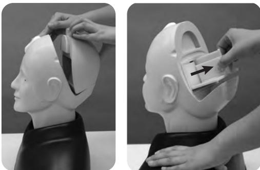
1. Remove the head cover on the back of the head.
