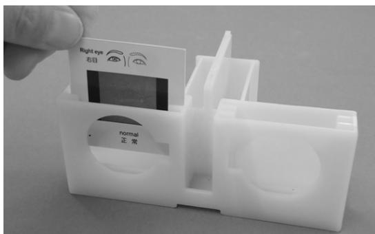
Do not touch the area of fundus image on the card directly, as fingerprints deteriorate the image quality and they can be unremovable. When handling the image cards, always hold the area of the white frames. For removing the dust on their surface, use the included blower.
