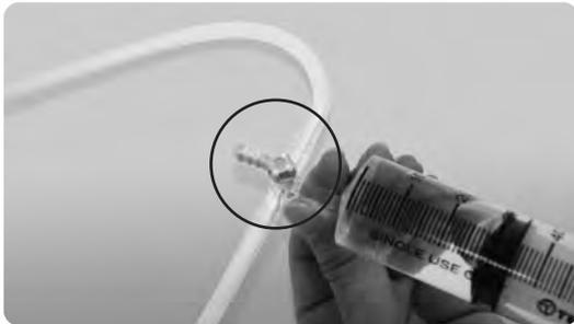
3. Flush out the inside of the airway unit with running water through each opening.
