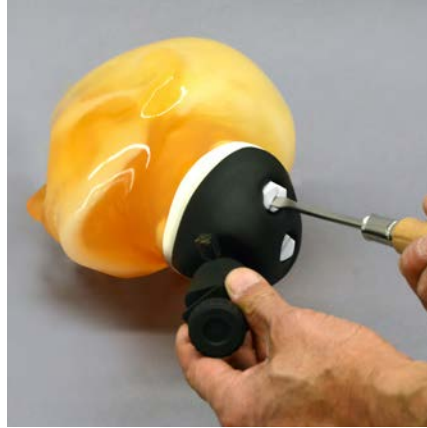
25 Screw bolt for neck connection M8x15x2
