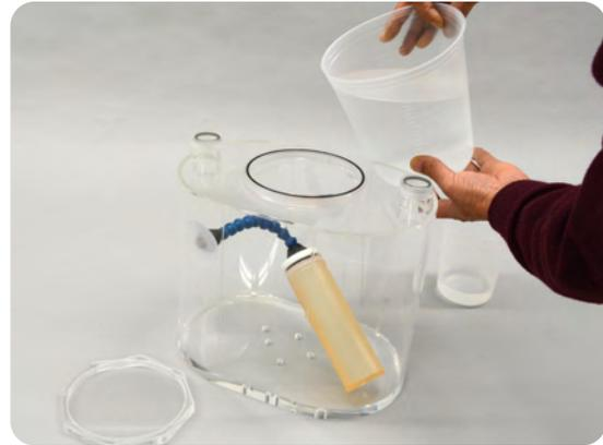
5. After covering container, open the two small caps to discharge the air remained by tilting the container, and fill it with water again.
