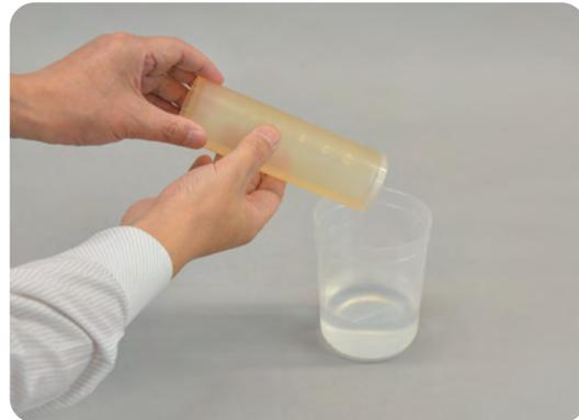
3. After covering colon unit, insert it to the hole where you need image. If you need another colon unit for image, repeat 1-2 process to prepare, and insert it to the hole.
