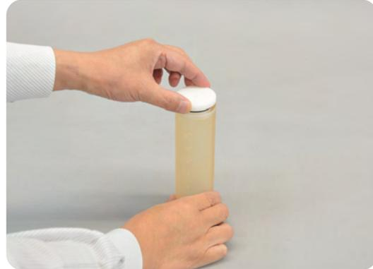
2. Tilt and rotate the colon unit slowly to coat the contrast agent throughout the inside of colon unit. Open colon unit again to drain the contrast agent.
