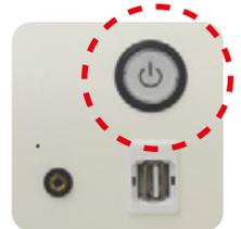
Once the light for the simulation power button changes to dim blinking, turn off the electricity power switch to the "O" mark, and plug out the power cable.
