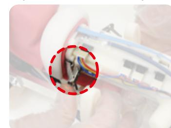
5. Insert the cable from the new tongue part to the terminal.
