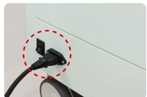
! Turn off the power before start replacing any parts.
