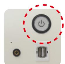
Once the light for the simulation power button changes to dim blinking, turn off the electricity power switch to the "O" mark, and plug out the power cable.
