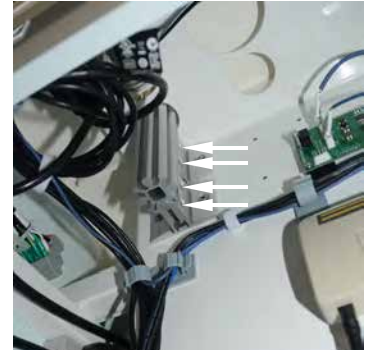
3, Open the back wall of the simulator unit. Loosen the four hexagon bolts with the wrench that fix the lower end of the pole.
