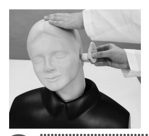
Insert the ear into the opening as shown in the photo below.
