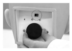
The cases can be switched by turning the switch dial. The number appearing in the window indicates the chosen case. Refer to the table on the quick manual. To practice foreign body removal, set the dial to "FB" and set the "FB Ear" type of external ears. Otherwise, you may damage the ear drum images and permanent alarm goes off.
