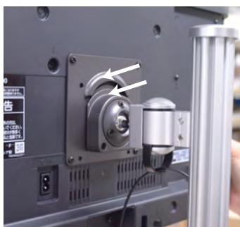
1. Put the metal fitting at the back of the monitor over the fitting at the head of the supporting arm.
