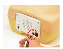
2. Connect reverse side of AC adapter to power socket.
