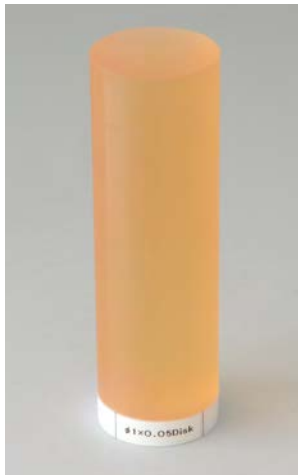
Bead phantom tungsten bead 0.3mm dia.
