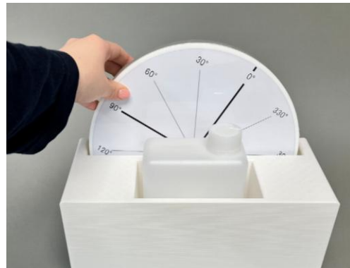
Turn the phantom to set a layout for imaging
