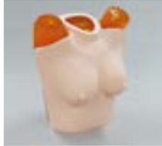
**Breast plate for Chest Phantom N-1 "LUNGMAN"**. This plate simulates the absorption of breast in female chest X-ray, and the influence of nipple on image quality.
