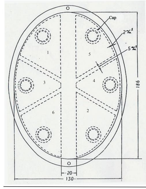
C) Section Phantom:6 fill/drain portsAcrylic resin (Transparent)
