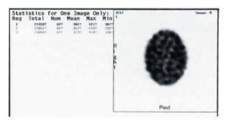
1-3-4. Non-uniformity in SPECT image highly depends on the non-uniformity in sensitivity of each scintillation camera itself. Such non-uniformity in a camera's sensitivity leads to ring artifacts in SPECT images; therefore it is important to keep its relative non-uniformity within 3%.
