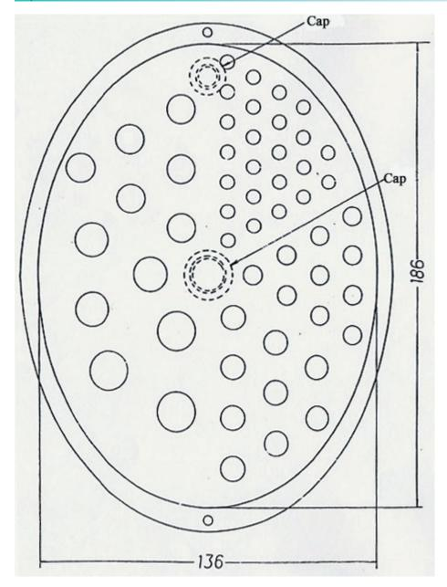
C) J-Jack Phantom:1 pair of fill/drain portsAcrylic resin (Transparent)
