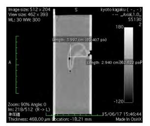
Bone scatterer case 258×158×H90mm Oval shape Shell thickness 10mm
