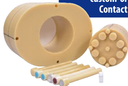
Multi Energy CT Quality Assurance Phantom Phantom for quality assurance. A variety of research samples can be inserted using small containers.
