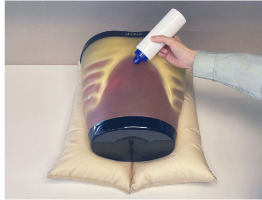
2. Spread lubricant gel on the phantom body.
