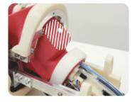
2. Connect the cable from the new sensor unit into the terminal.
