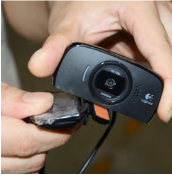
1, Open the lid of the camera. Rotate the camera head 180 degrees and fold back the lid.
