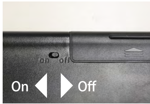
2, Turn on the switch at the back of the keyboard.
