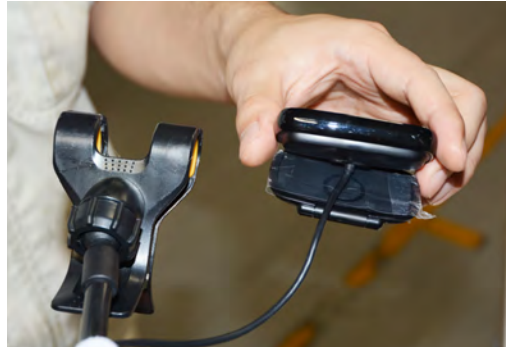
2, Hold the camera by the clip at the top of the camera arm on the pole.
