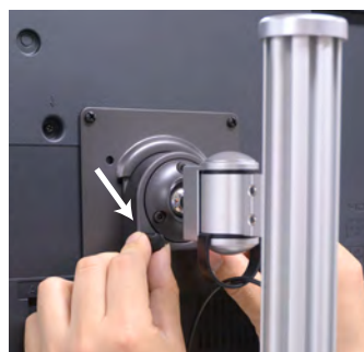
2. Fix the fittings with two screws.
