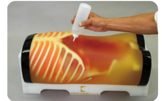
2. Spread ultrasound gel over the phantom body.
